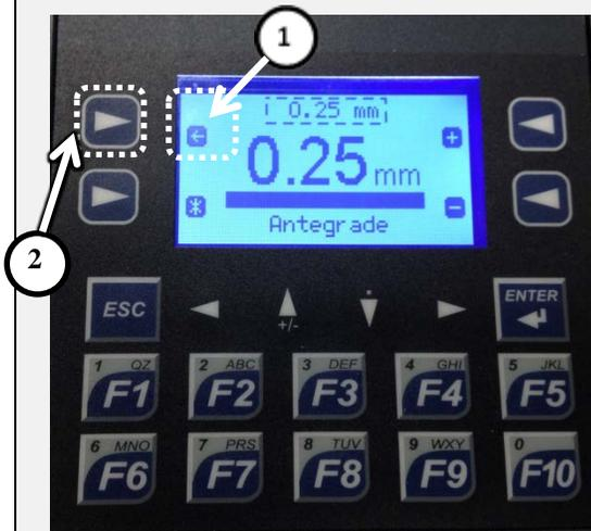
1 After you have completed lengthening, the arrow on the display next to the top left key will flash.
